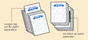
The printer separates tags by cutting the first tag longer or using the ink roller mechanism to place an ink mark on the side of each batch separator tag.
