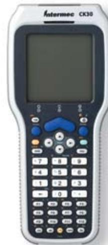
**Three distinct keypad options ranging from the simplified 42-key to a full 52-key alphanumeric offer layouts for a range of applications.**
