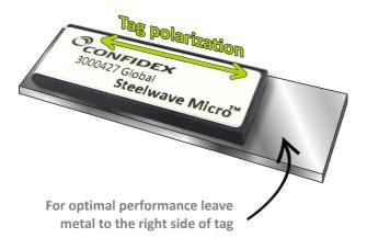
To achieve the optimal performance please locate the tag on metal like shown above. Ideally the tag is placed on large even metal surface with direct metal contact underneath the whole tag.
